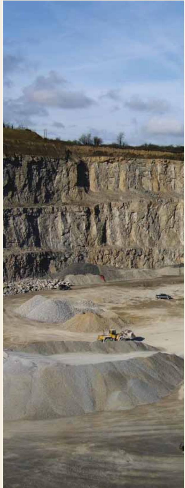
Piles of crushed rock aggregate ready for use are stockpiled on the quarry floor
